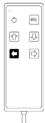
Figure 18 - RTC Button on Hand Control
