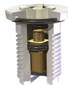
The air jets on the Air Spa System feature spring loaded check valves for back flow prevention, which eliminates the extra step to disinfect the air lines.
